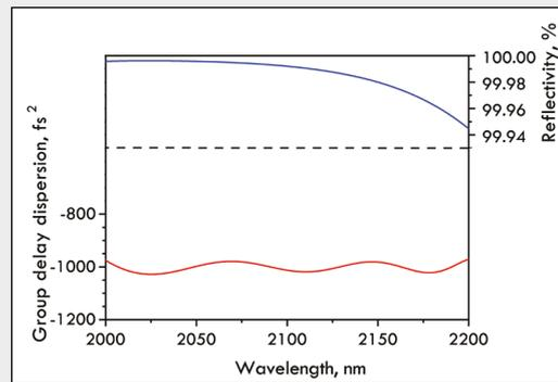
*Infrared dispersive mirrors with negative GDD: PC1741 (left) and HD1501 (right).*
