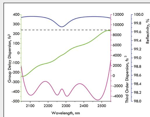
*Infrared dispersive mirrors with TOD: IR1304\_RC2 (left) and TOD1601 (right).*
