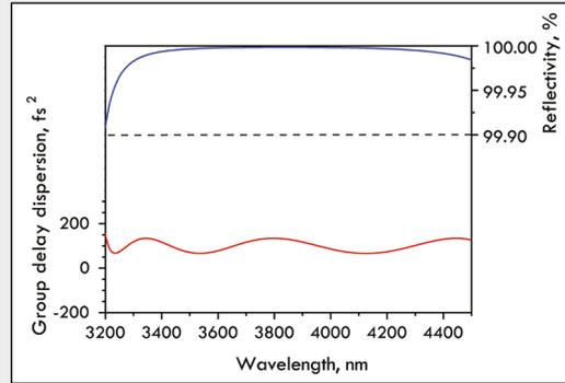
*Infrared dispersive mirrors with positive GDD: IR1402 (left) and HD1715 (right).*
