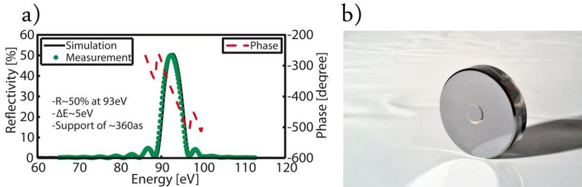
Figure 2: a) Simulation and XUV reflectivity measurement, together with the simulated phase evolution, for the XUV93eVBW5eV mirror design, supporting  $\sim 360$  as pulses. b) Image of a coated XUV double mirror with a core diameter of 5mm for e.g. IR/XUV time delay experiments being used for attosecond streaking.
