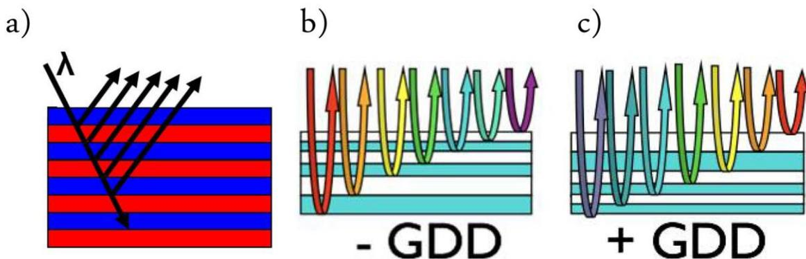
Figure 1: a) Physical principle of a XUV multilayer mirror for a strong periodic mirror, enabling a nearly gaussian reflectivity and nearly chirp free spectral phase. In case of necessarily phase corrections one can use aperiodic mirrors introducing a negative group delay dispersion b) or a positive one c).
