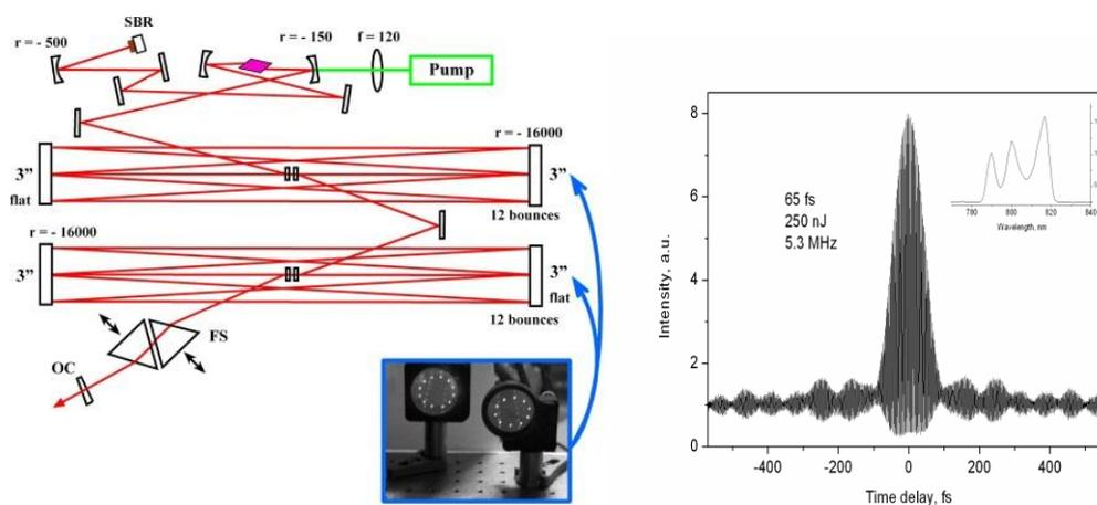
Fig. 1. Left: cavity configuration of the 5-MHz Ti:sapphire CPO. Insert: the beam spots on the DMs forming the delay line. All radii are given in mm. SBR: saturable Bragg reflector; FS: fused silica prisms for fine tuning intracavity GDD, OC: output coupler. Right: the autocorrelation trace of the generated pulses compressed by another set of (different) chirped mirrors external to the cavity (not shown). Inset: the generated spectrum.
